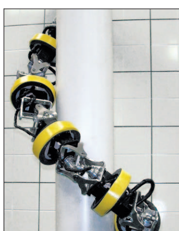
HyDRAS, a robot whose name stands for Hyper-redundant Discrete Robotic Articulated Serpentine for climbing, is able to crawl up a pole by converting the oscillating motion of its joints to a whole-body rolling motion.
